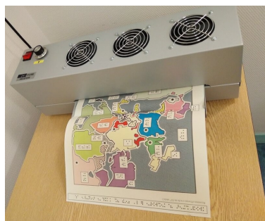
Illustration 30: Production of a thermo- inflated drawing
