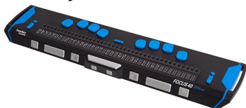
Illustration 23: The Braille display, keyboard and terminal
